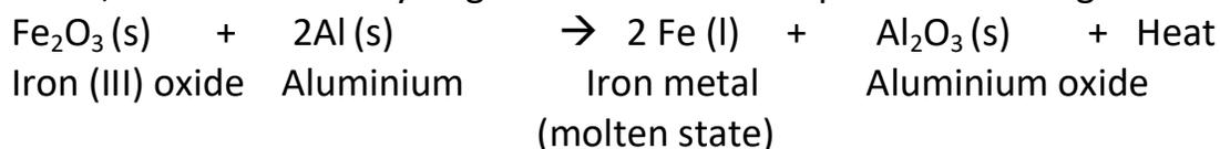
The heat gives out in this reaction is so great that iron metal formed by this reaction is in molten state. This molten iron can be poured b/w broken rail pieces (or other broken iron objects) to weld them together.
